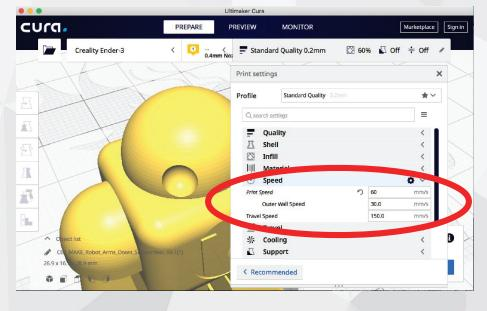
Here we choose to manually set the three speeds circled in red also to highlight how they are different from each other. The first of them, "Print speed", is the reference value that the software needs to calculate all the speeds in the various phases, except for the other two that we will set manually.
