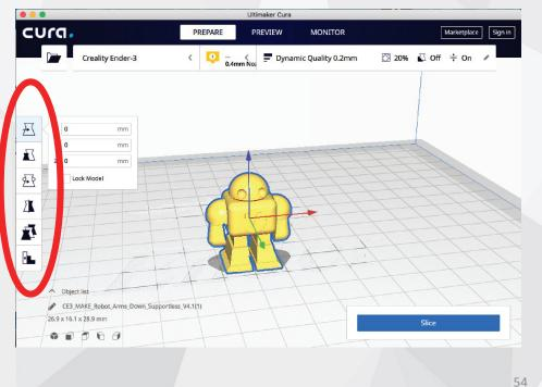
The first icon at the top will activate the function of moving the model, in three directions: X, Y and Z. By default, the model is positioned in the center; it will be moved only if needed (eg simultaneous printing of several objects)
