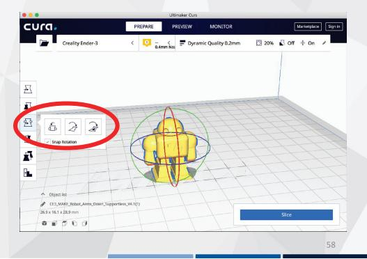
The fourth icon activates the mirroring function of the model, useful when the model has no symmetry plans and you want to obtain a mirrored model, for example a "left" if you have a "right".
