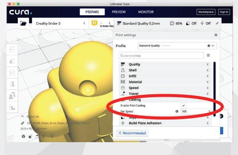
The software, automatically, activates the cooling after the second layer, in order to guarantee that the first layer has an optimal adhesion to the printing bed. With tricky materials, such as ABS or Nylon, it may be necessary to deactivate the cooling or reduce the fan speed.
