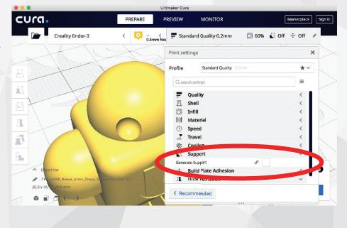
To better understand the importance of the supports, let's look at the areas circled and indicated by the arrows in the figure: what happens when the printer extrudes the material to generate those areas? Without an underlying support, the molten material would run down, at least until it remains fluid.
