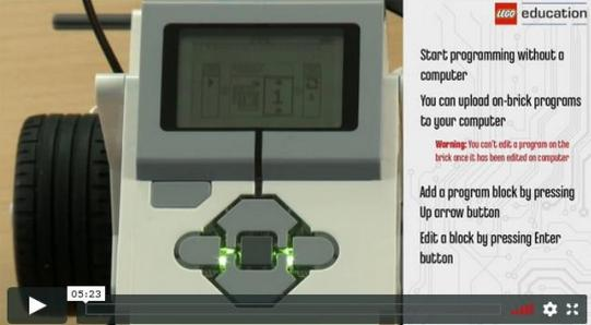
You can program the EV3 using the on-brick applications. Now, you can program the brick directly without the need for a computer. This is especially useful when out in the field.
