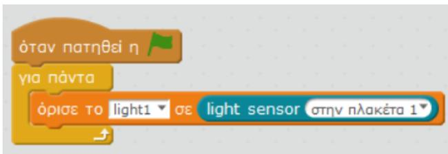
Connect the robot and press the green flag. You will notice that the light sensor values are displayed in the variable light1. If you cover the light sensor 1 with your hands, you will notice that the value of the light1 variable in the upper left corner of the scene is constantly changing. The closer your hand is to the light sensor, the less light the sensor detects, so the value of the variable will be lower.
