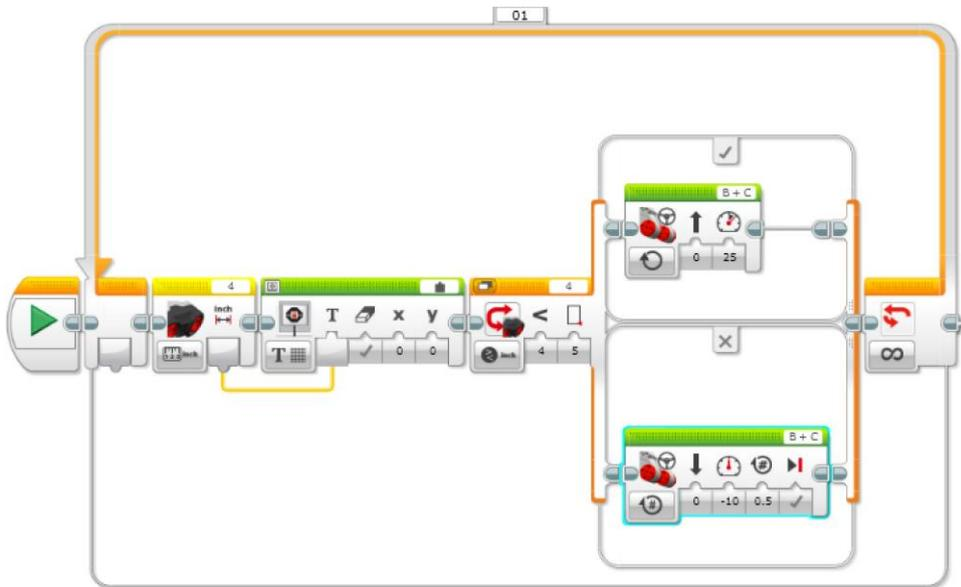
**Learning objectives:** Students will build and program the robot so that it is able to stay on a table without falling off. Concepts covered: Ultrasonic sensor, “Display” block.
