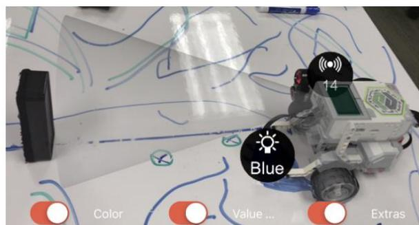
**Figure 3:** A view from our existing application showing two types of sensory data of the EV3 robot: 1) the sonar reading, shown as a cone and also as a number (14 cm) indicating the distance to the object; and 2) the color reading (in this case, Blue)
